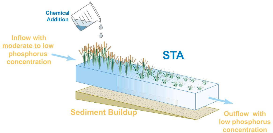
**Figure 4C-16.** Schematic representation of the low intensity chemical dosing advanced treatment technology tested at north STA-1W Test Cell Research Facility.
