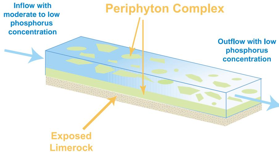
**Figure 4C-8** Schematic representation of the periphyton vegetation advanced treatment technology tested at STA-1W.
