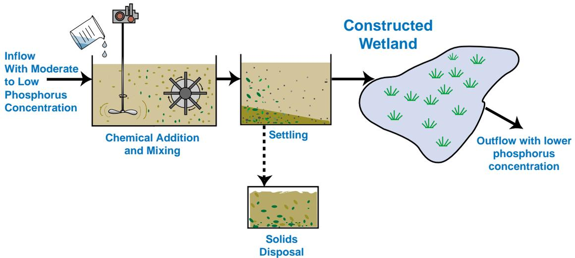
**Figure 4C-13.** Schematic representation of the managed wetland advanced treatment technology tested at the north and south STA-1W Test Cell Research Facilities.
