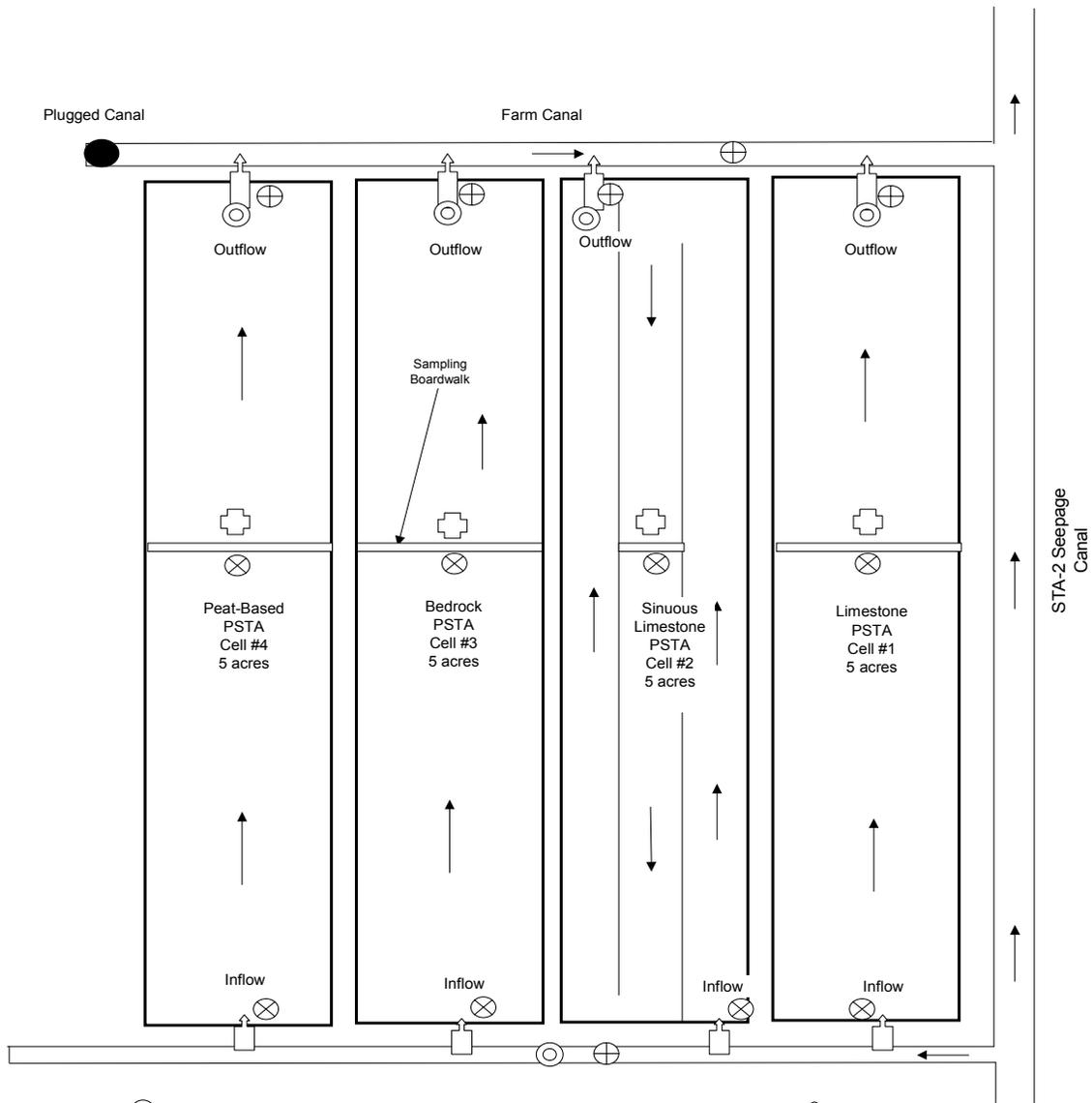
**Figure 4C-12.** Periphyton Stormwater Treatment Area 20-acre field site schematic. The site is located along the western edge of STA-2.
