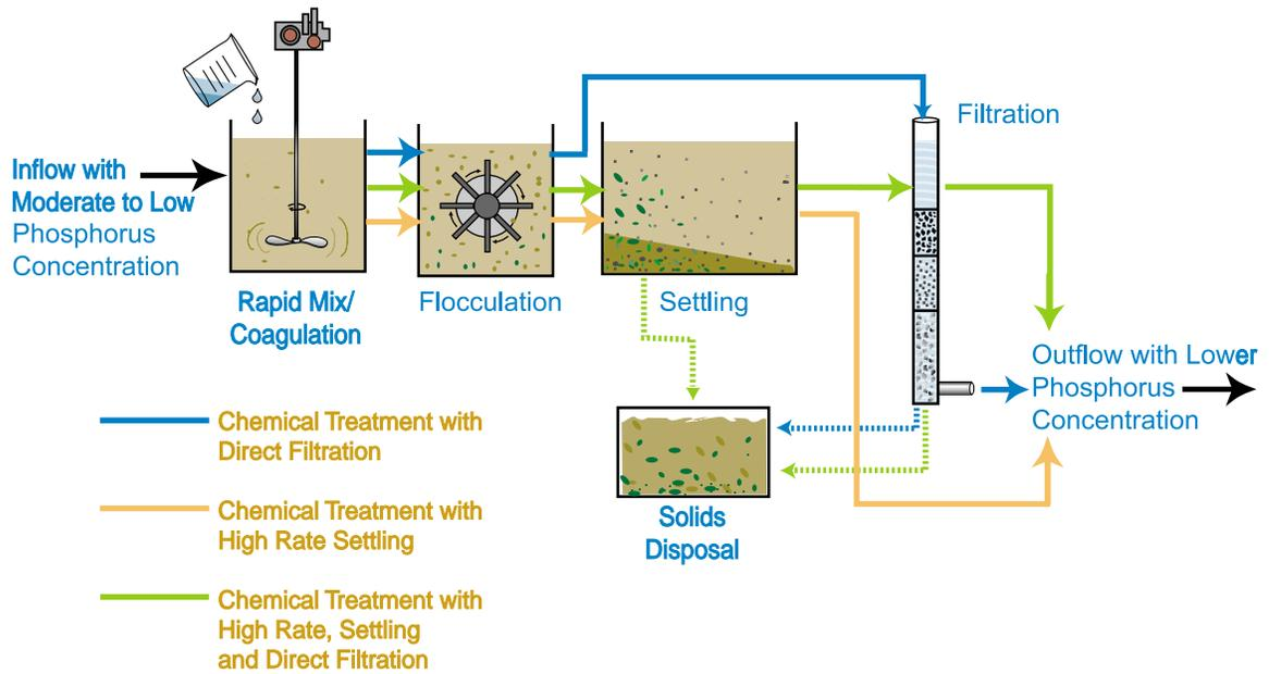
**Figure 4C-21.** Schematic representation of the chemical treatment followed by solid separation advanced treatment technology tested at STA-1W Post-BMP and Post-STA research sites.
