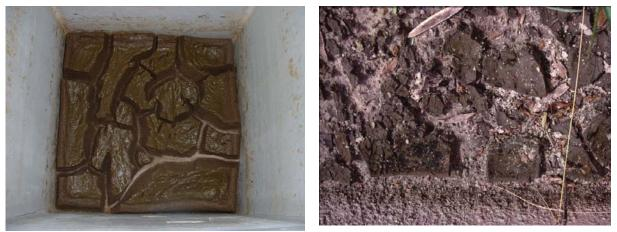
Figure 3. Alum Floc Drying Process.
