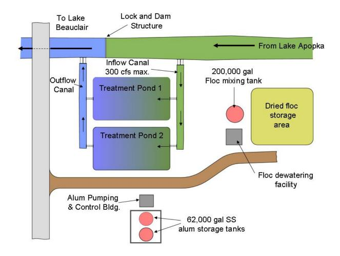
Figure 1. Schematic of Lake County NuRF Facility.
