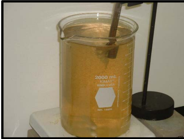
Immediately after alum / polymer addition
