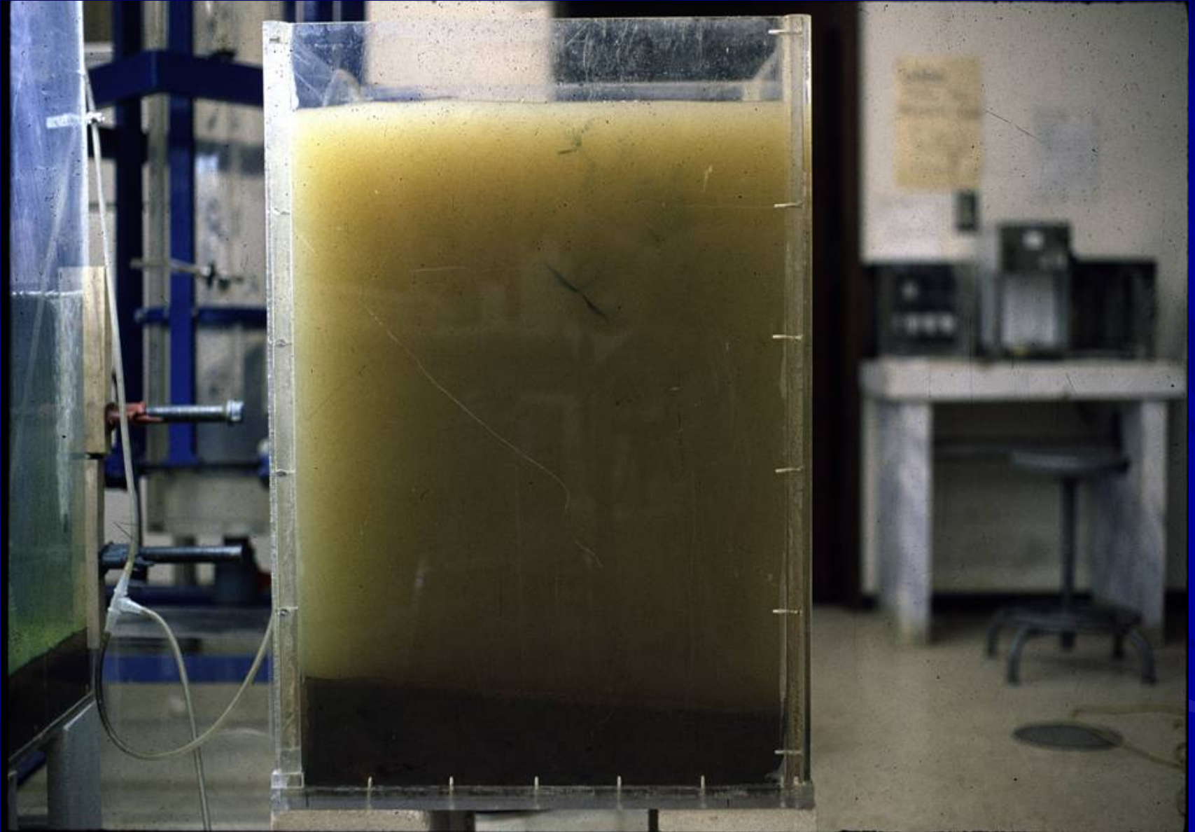
Colloidal Runoff Sample Settled for 45 Days
