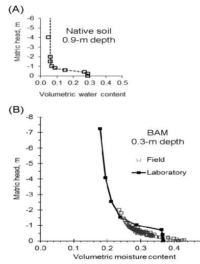
Field measurements were obtained by continuous monitoring using time domain reflectometry and tensiometers.
