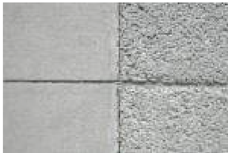
Figure 1.1.2 Comparison of Conventional Concrete and Pervious Concrete
