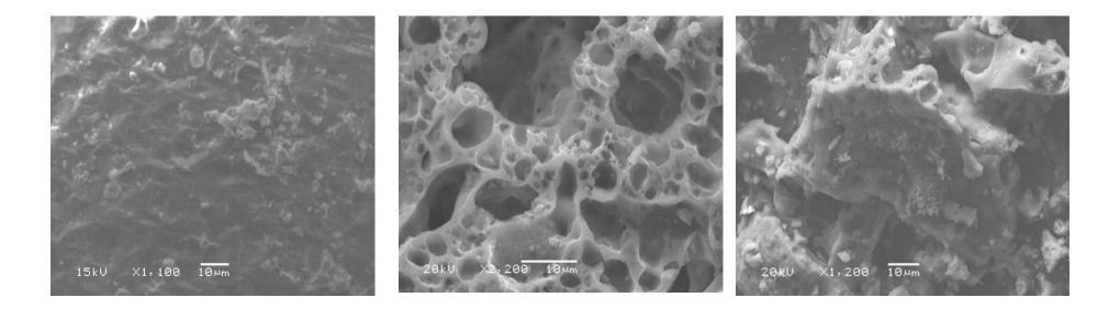
SEM of (*a*) concrete sand1,000 x, (*b*) expanded clay 2,200 x, and (*c*) tire crumb 1,200 x magnification showing the surface structure and characteristics after residing in 24 days of column testing.
