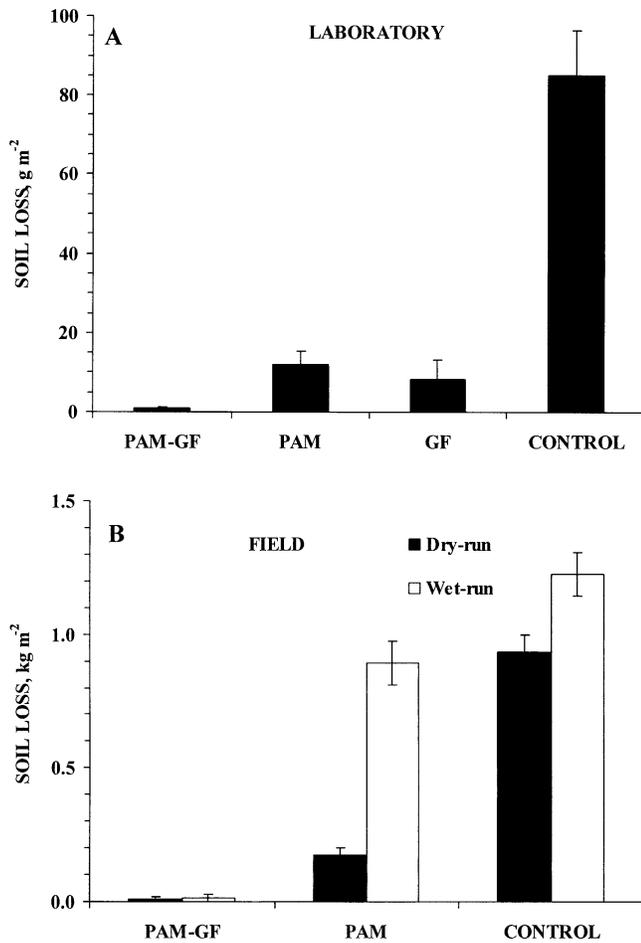
Fig. 1. Mean soil loss on an event basis from soil berms treated with polyacrylamide (PAM), geotextile fabric (GF), and PAM plus GF (PAM-GF), and a control berm without PAM or GF; (A) laboratory and (B) field for the dry and wet run rainfall simulations. Error bars represent standard deviation of the mean ( $n = 3$ ).
