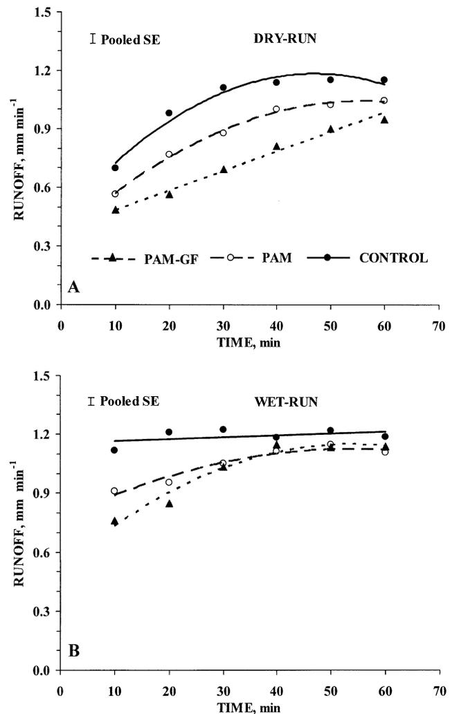
Fig. 4. Mean runoff within the event from soil berms treated with polyacrylamide (PAM), PAM plus geotextile fabric (PAM-GF), and a control berm without PAM or GF under field conditions for the (A) dry- and (B) wet-run rainfall simulations. Error bars represent the pooled standard error of the treatment means ( $n = 3$ ).
