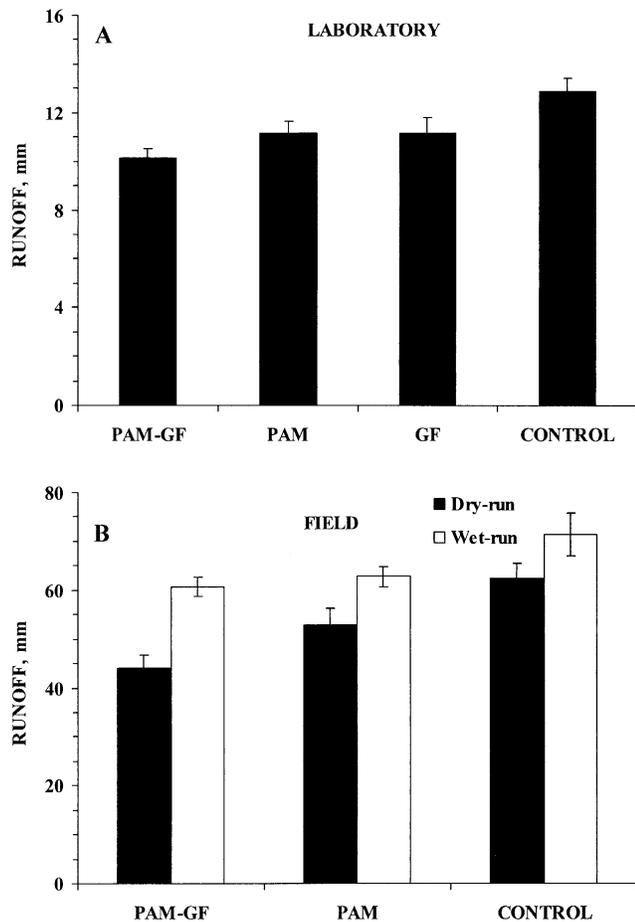
Fig. 3. Mean runoff on an event basis from soil berms treated with polyacrylamide (PAM), geotextile fabric (GF), and PAM plus GF (PAM-GF), and a control berm without PAM or GF using simulated rainfall; (A) laboratory and (B) field. Error bars represent standard deviation of the mean ( $n = 3$ ).
