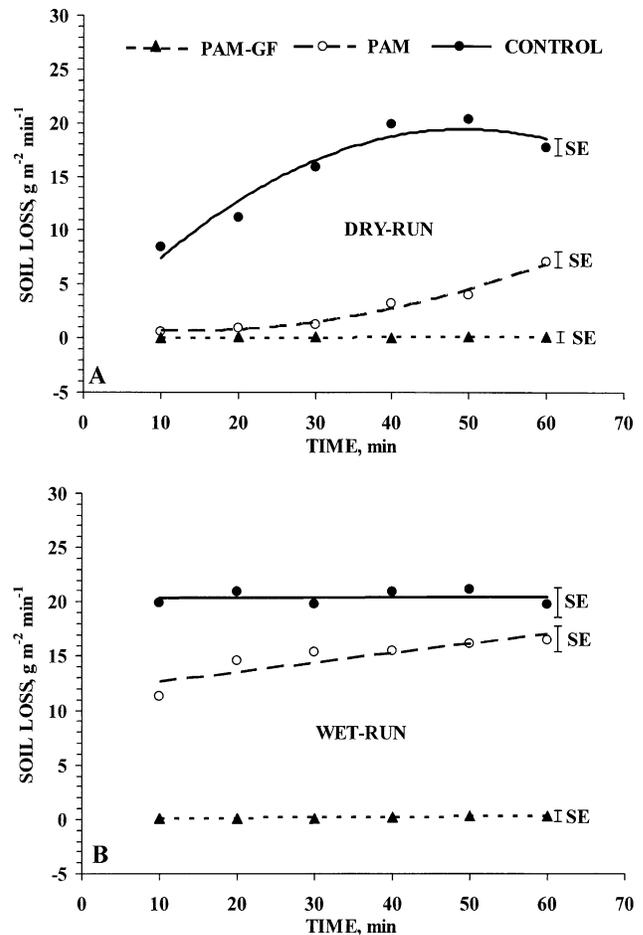
Fig. 2. Mean soil loss within the event from soil berms treated with polyacrylamide (PAM) and PAM plus geotextile fabric (PAM-GF), and a control berm without PAM or GF under field conditions for the (A) dry and (B) wet run rainfall simulations. Error bars represent the pooled standard error of the treatment means ( $n = 3$ ).
