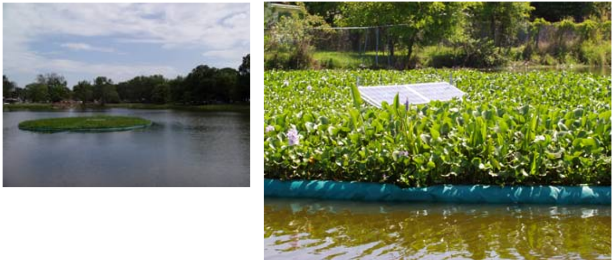
Figure 1. The floating wetland deployed in Lake June. The photo on the right depicts a closer view of the solar panels and vegetation.
