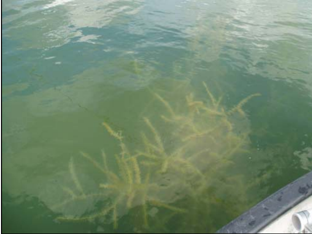
Figure 1. Coagulant floc attached to submerged macrophytes near the inflow region of a HWTT system.
