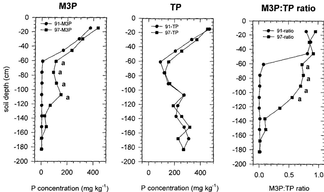
Fig. 2. Mehlich 3 phosphorus (M3P), total phosphorus (TP), and ratio of M3P to TP extracted from three soil profiles collected from the spray field in 1991 and 1997. Points followed by the letter *a* are significantly different at  $P < 0.1$ .
