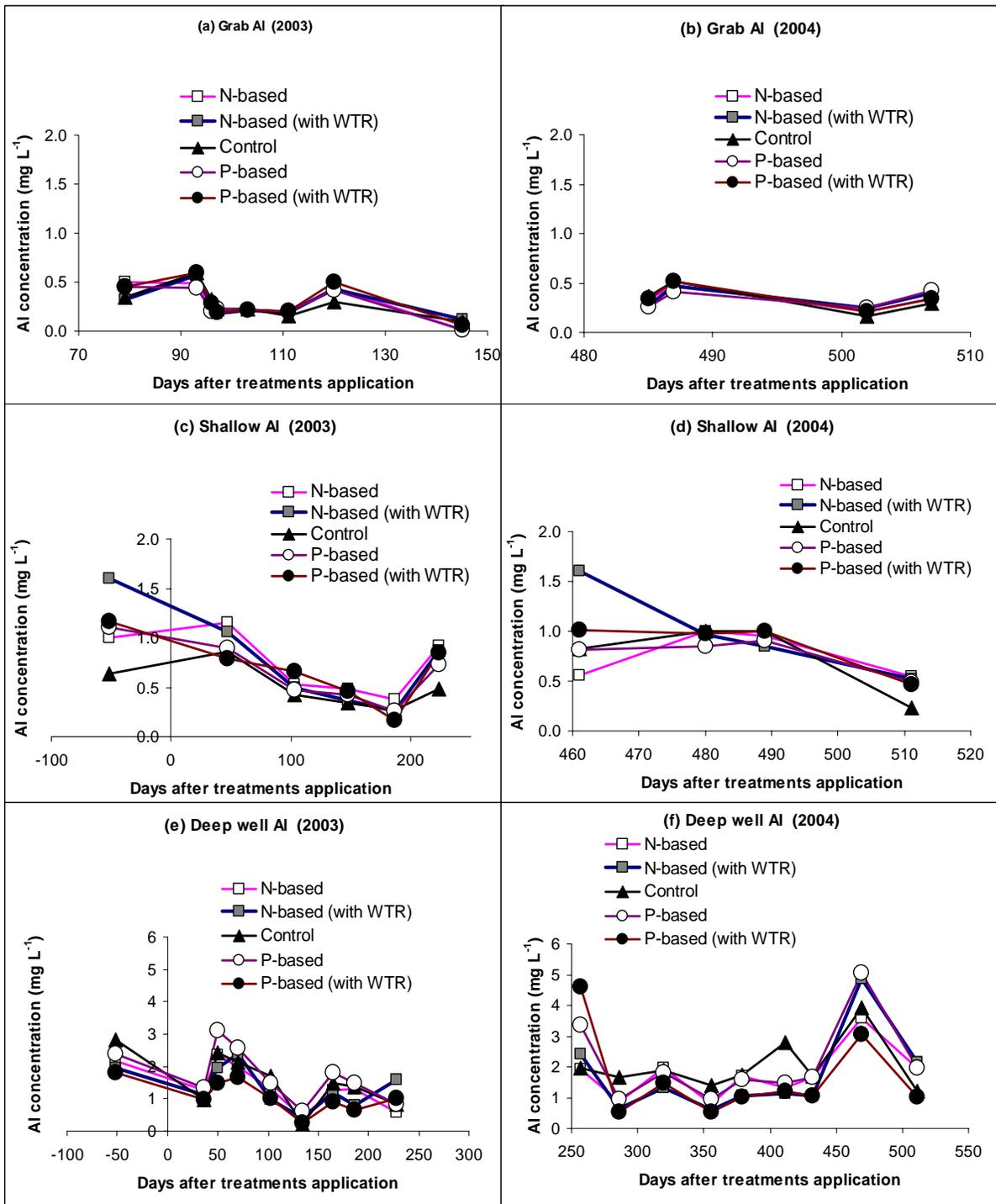
Figure 9-5. Trends of AI concentrations surface grab (a and b), shallow well (c and d) and deep well (e and f) water samples taken during the study.
