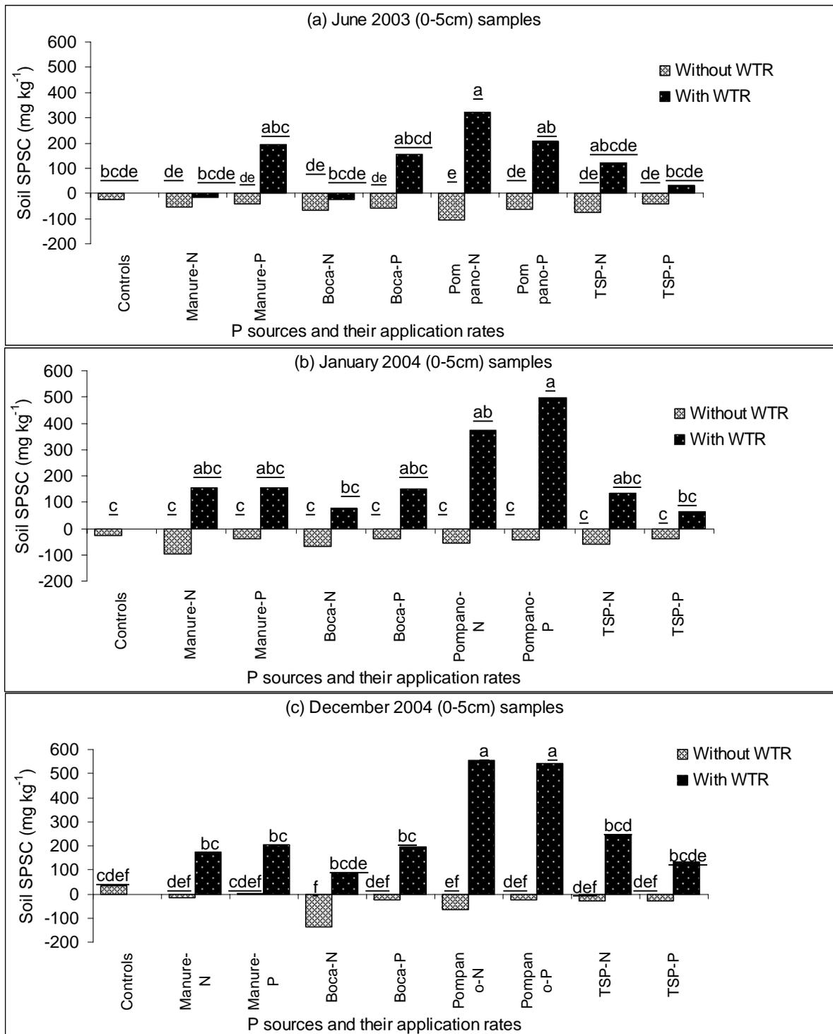
Figure 4-8. Soil phosphorus storage capacity (SPSC, mg kg<sup>-1</sup>) values of A-horizon (0-5cm) samples from the field study (June 2003 – Dec. 2004) as affected by the treatments. (Treatments ending in P, and N, are P-based and N-based rates of the sources, respectively). Treatments with the same letters are not different at  $p = 0.05$  by Tukey test.
