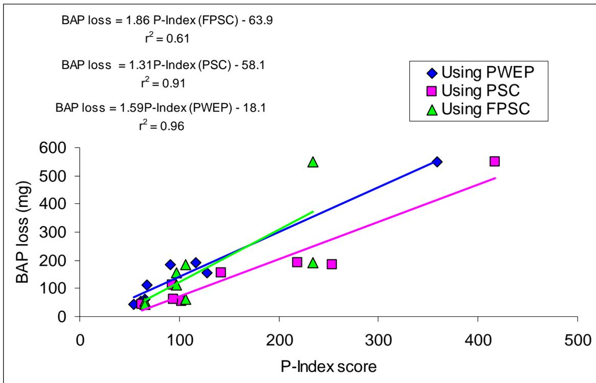
Figure 8-2. Regression of bioavailable P (BAP) loss with P Index score obtained using varying measures of coefficients (Percentage water extractable P (PWEP); P-source coefficients (PSC); Florida P Index source coefficients (FPSC)).
