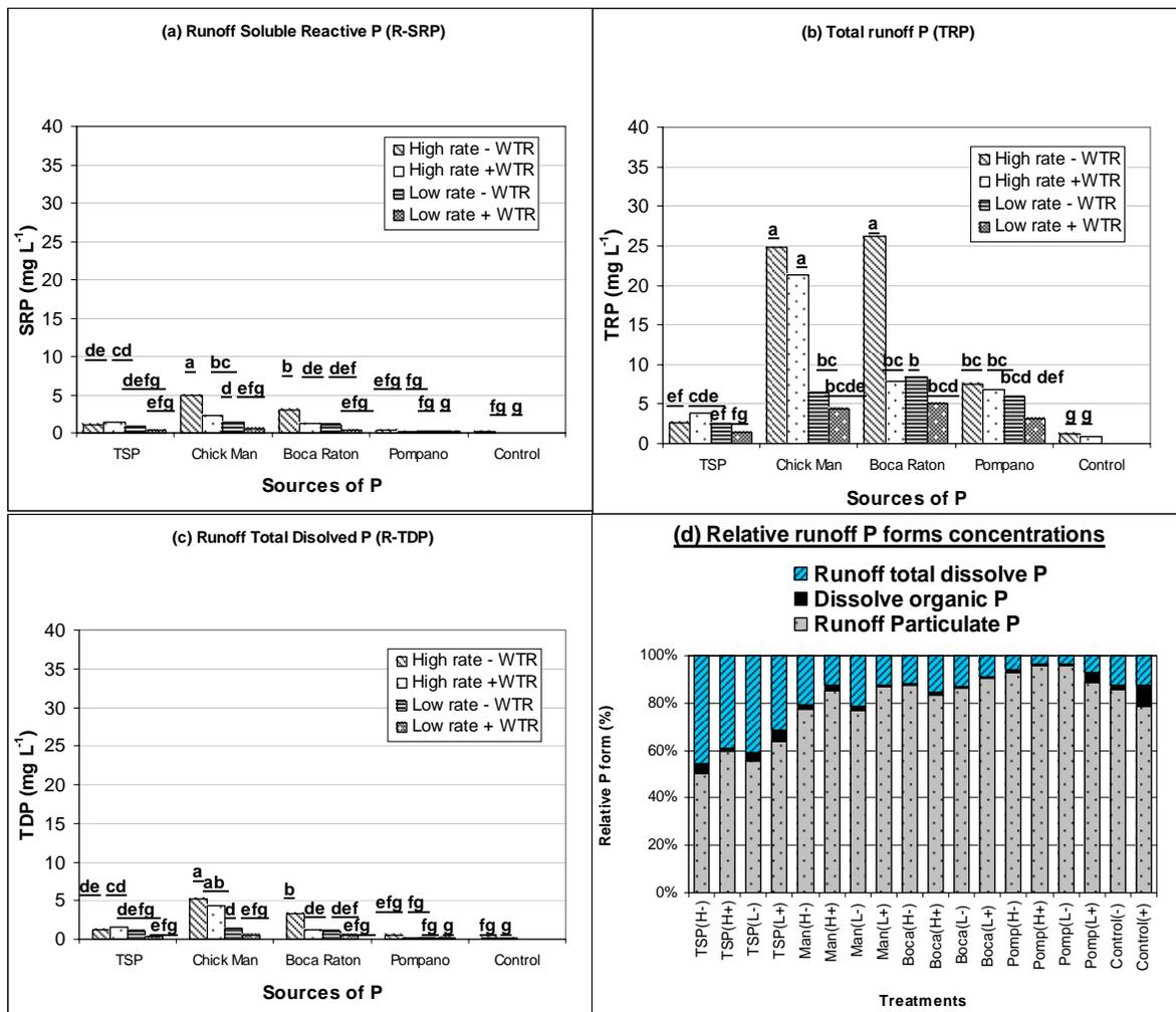
Figure 7-3. Runoff flow-weighted mean (a) soluble reactive P (b) Total P (c) Total dissolved P concentrations and (d) relative P forms concentrations for the various treatments (Treatments followed by the same letters are not different at  $p = 0.05$  by Tukey)
