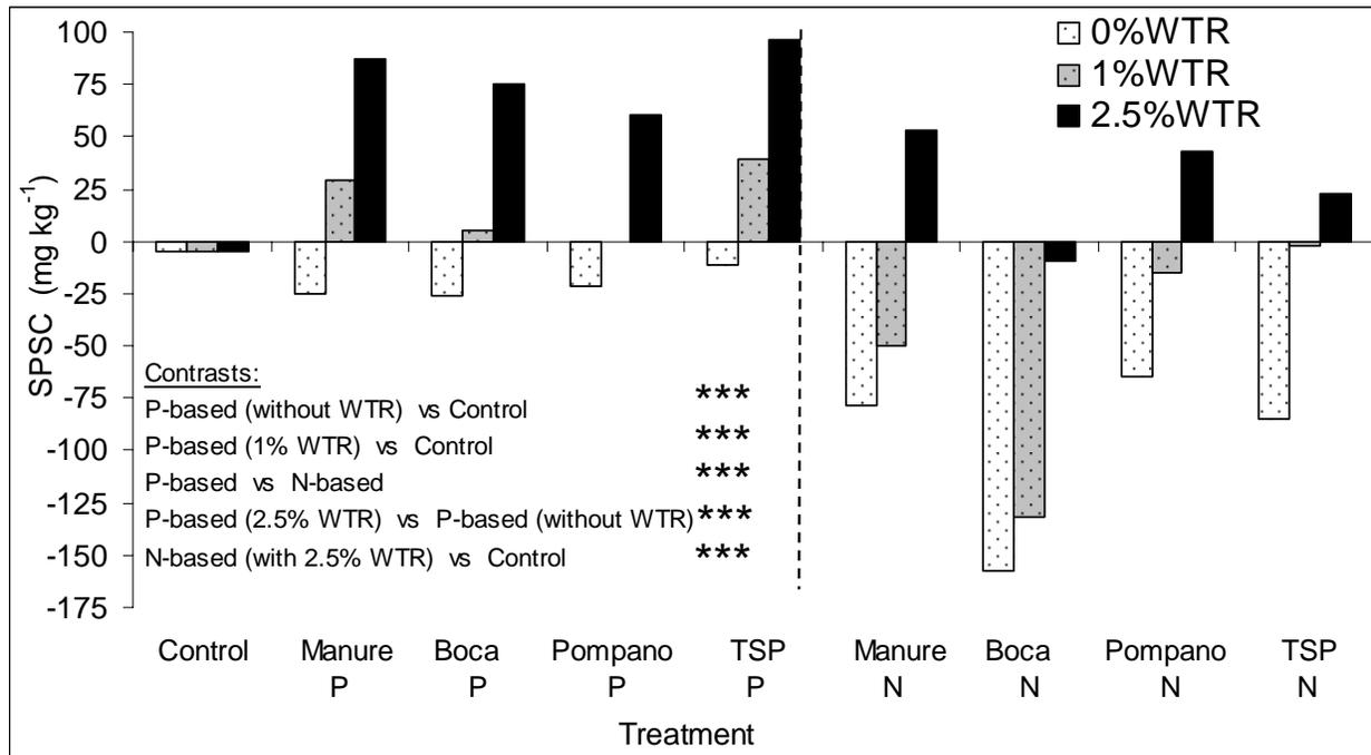
Figure 6-1. Soil phosphorus storage capacity (SPSC,  $\text{mg kg}^{-1}$ ) values for the different treatments in time zero samples taking during glasshouse study. (Treatments ending in P, and N, are P-based and N-based rates of the sources, respectively).
