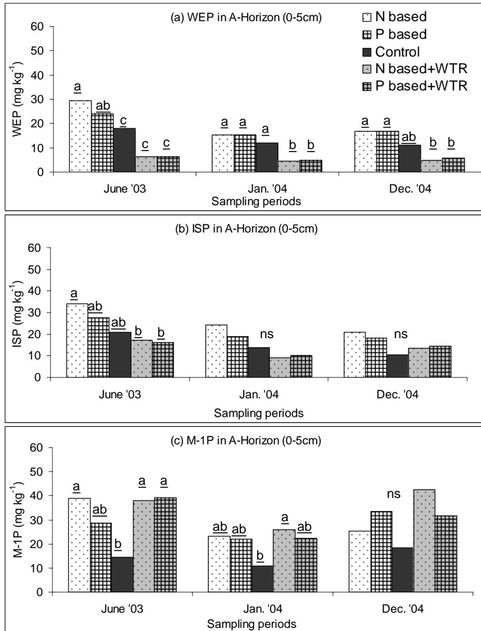
Figure 5-3. Effects of P-source rates and water treatment residual (WTR) on (a) water extractable P (WEP), (b) Iron strip P (ISP), and (c) Mehlich 1P (M-1P) values of A-horizon (0-5cm) soil samples taken during the field study.
