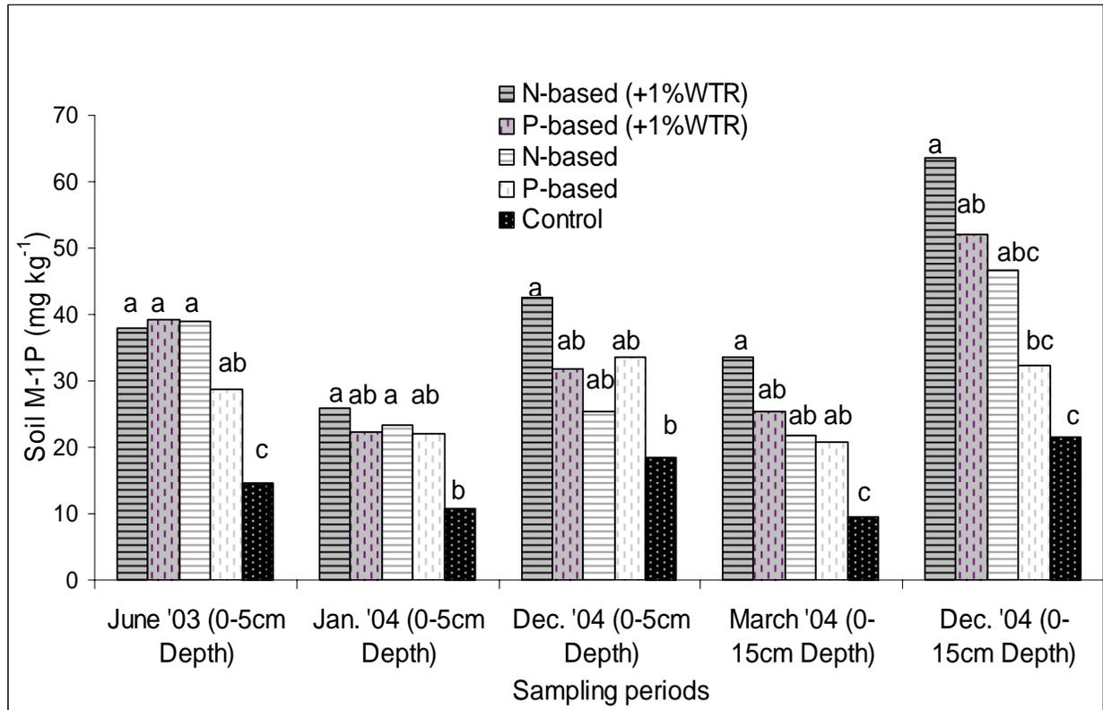
Figure 4-1 Effects of water treatment residual (WTR) rates and P-source rate on Mehlich 1 P (M-1P) values of A-horizon soils at each of the sampling periods ( $n = 12$ ). Treatments within the same sampling period with the same letters are not different at  $p = 0.05$  by Tukey test.
