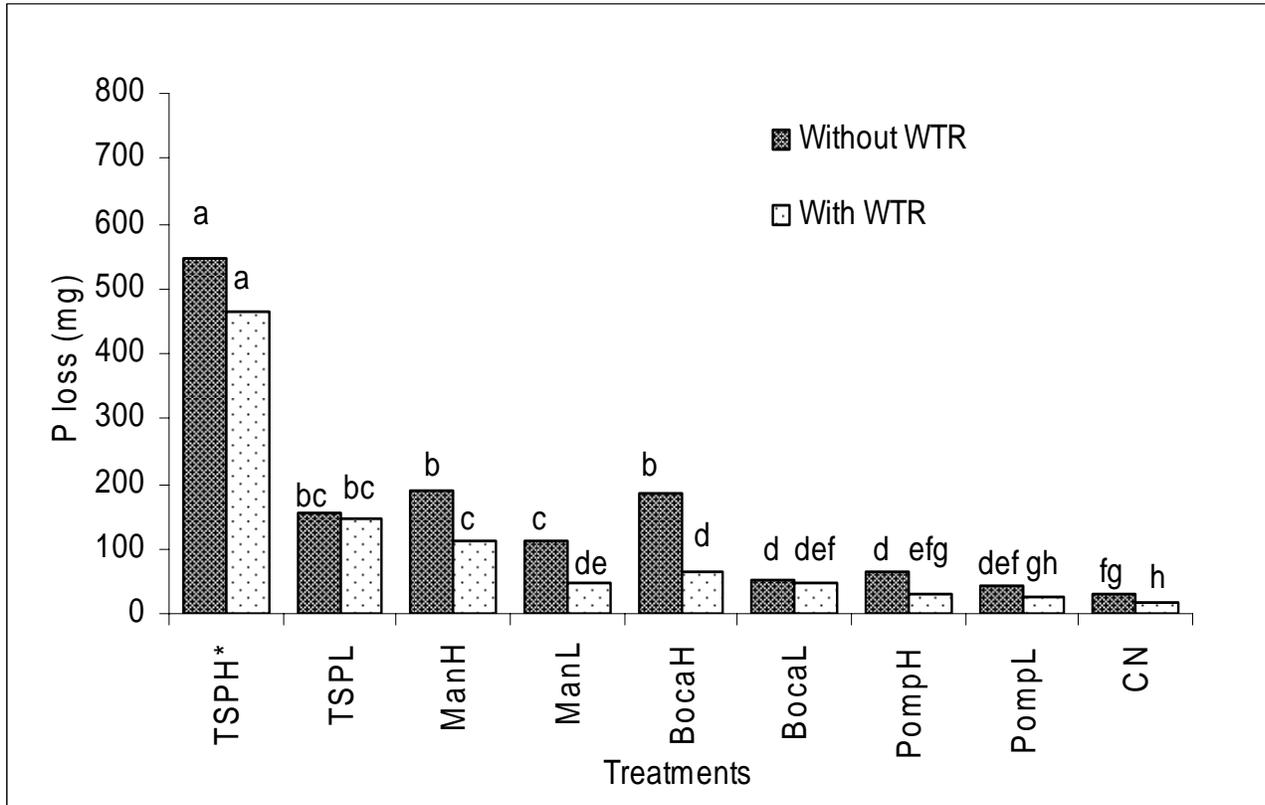
Figure 7-7. Total (runoff +leachate) mass of bioavailable P (BAP) lost during the three rain events. \*Treatments ending with ‘H’ and ‘L’ represents high and low application rate of the P-sources, respectively. (Treatments with the same letters are not different at  $p = 0.05$  by Tukey test)
