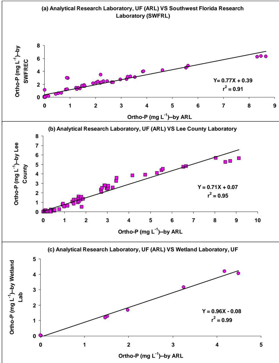
Figure 9-7. Regression of ortho-P concentrations results in groundwater samples reanalyzed by three other laboratories (UF-IFAS Southwest Florida Research Laboratory (SWFRL); Wetland Biogeochemistry Laboratory, UF; and Lee County Laboratory) with values obtained from Analytical Research Laboratory.
