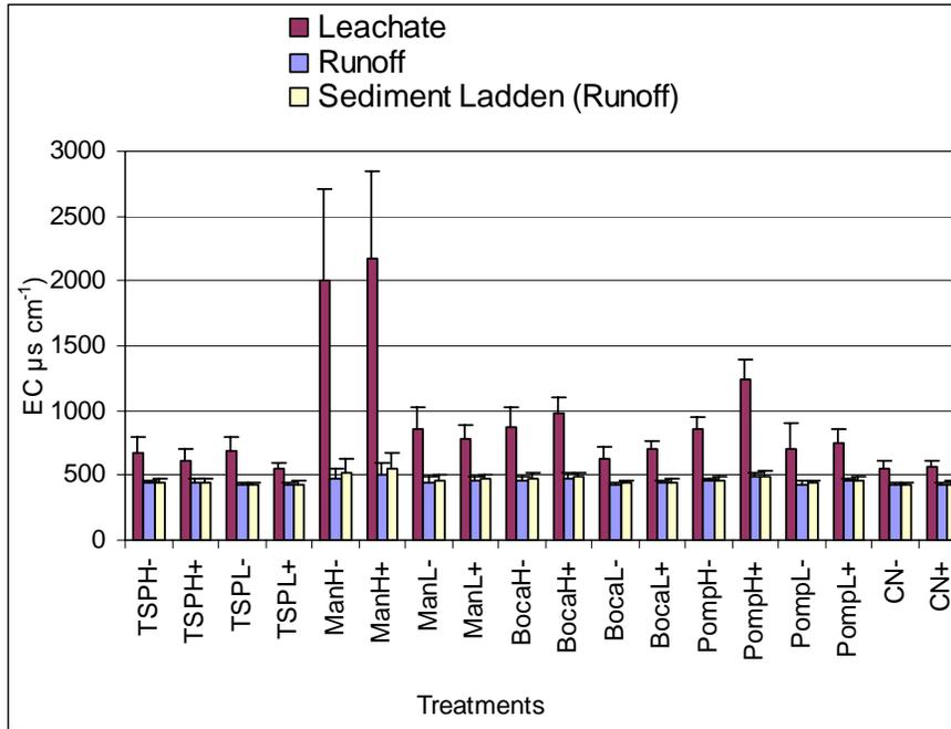
Appendix Figure B-5. Runoff and leachate EC values of the treatments across the three runs and replicates during the rainfall simulation experiment (n = 6, error bars represent one standard error)
