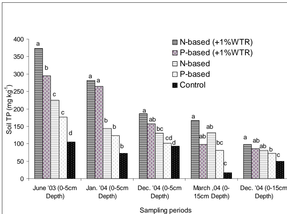
Figure 4-2 Effects of WTR rates and P-source rates on Total P (TP) values of A-horizon soils at each of the sampling periods. (Treatments within the same sampling period with the same letters are not different at  $p = 0.05$  by Tukey's test).
