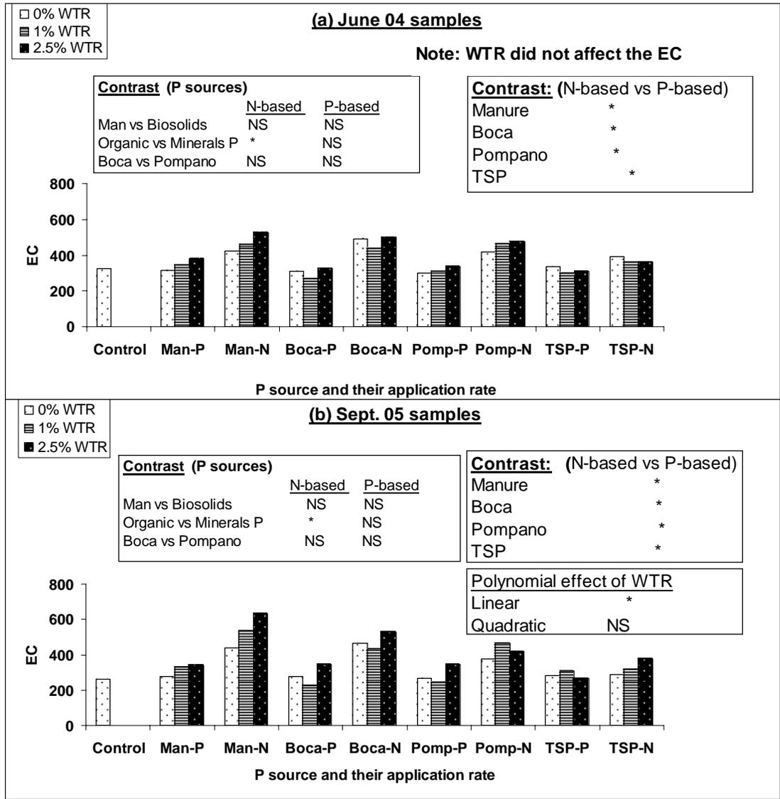
Appendix Figure B-2. The EC values ( $\mu\text{s cm}^{-1}$ ) of time zero and time final soil samples taken during the glasshouse study. (\* significant at 5%; NS is non significant at 5%)
