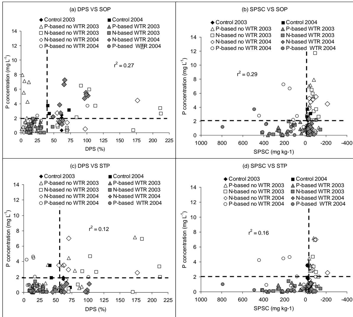
Figure 9-11. Relationships between soil P sorption indices (Degree of P saturation (DPS), and soil P storage capacity (SPSC)) and shallow well water ortho-P (SOP), and Total dissolved P (STP) concentrations.
