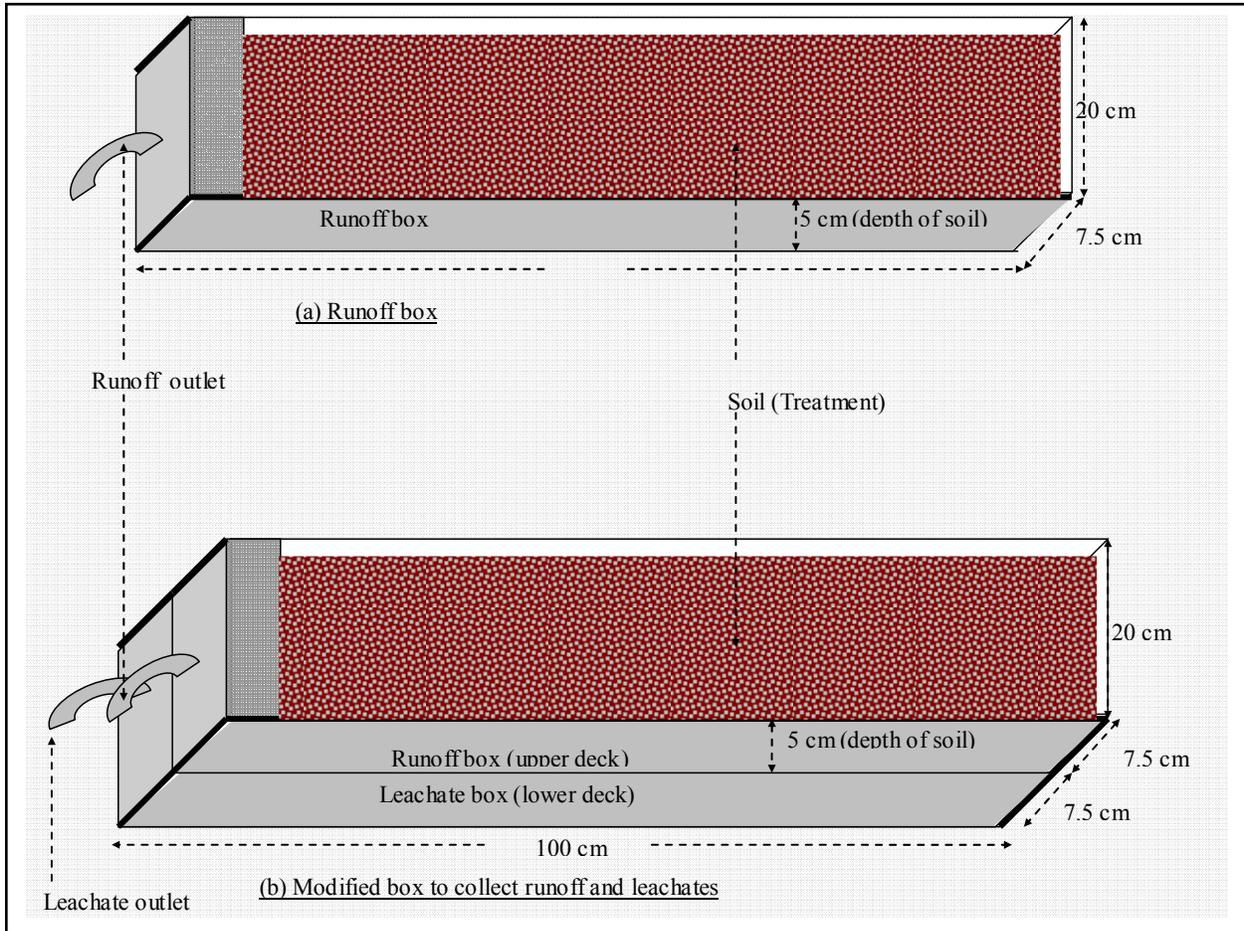
Figure 7-1. National P Research project (a) runoff box design and (b) box design modified to collect runoff and leachate simultaneously.
