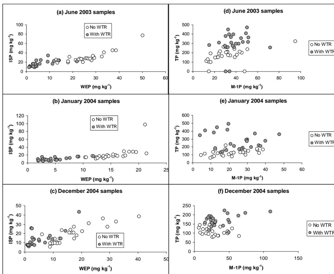
Figure 5-6. Relationships between water extractable P (WEP) and iron strip P (ISP) of (a) June 2003, (b) January 2004, (c) December 2004; and between Mehlich 1 P (M-1P) and Total P (TP) values of (d) June 2003, (e) January 2004, (f) December 2004 soil samples taken during the field study and the effects of water treatment residual (WTR)
