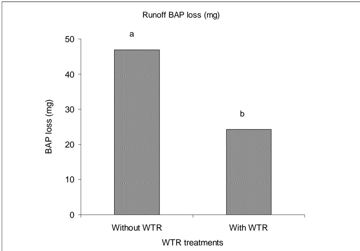
Figure 7-6. Effect of WTR on runoff BAP mass loss (Treatments with the same letters are not different at  $p = 0.05$  by Tukey).
