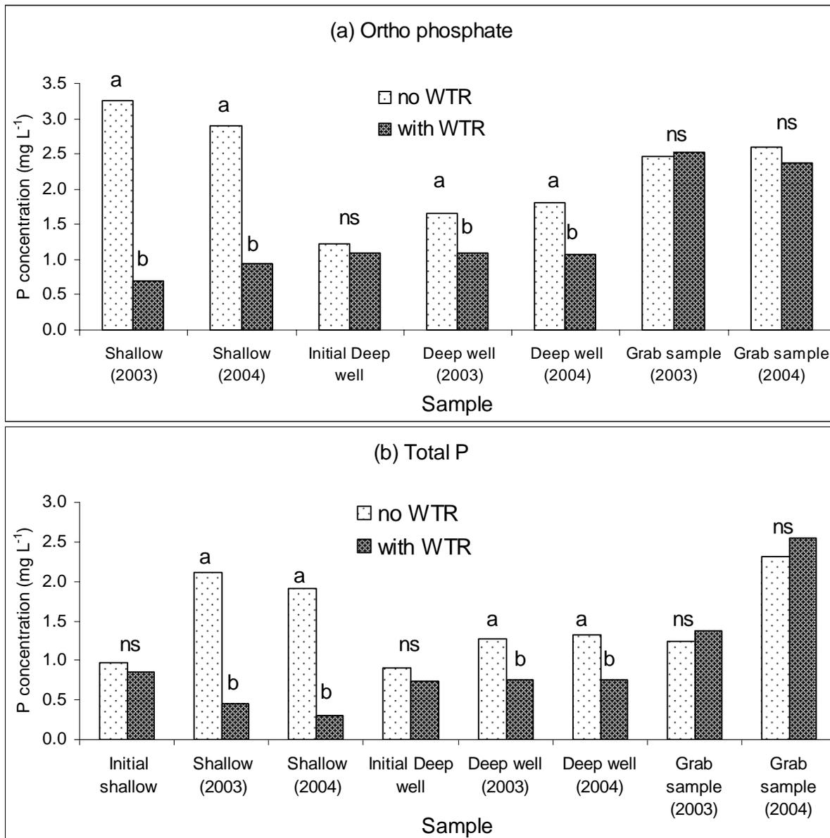
Figure 9-10. Total dissolved and Ortho-P concentrations of water samples taken during the study as affected by WTR application. Treatments bar within the same sampling period capped by the same letters are not different at  $p = 0.05$  by Tukey test
