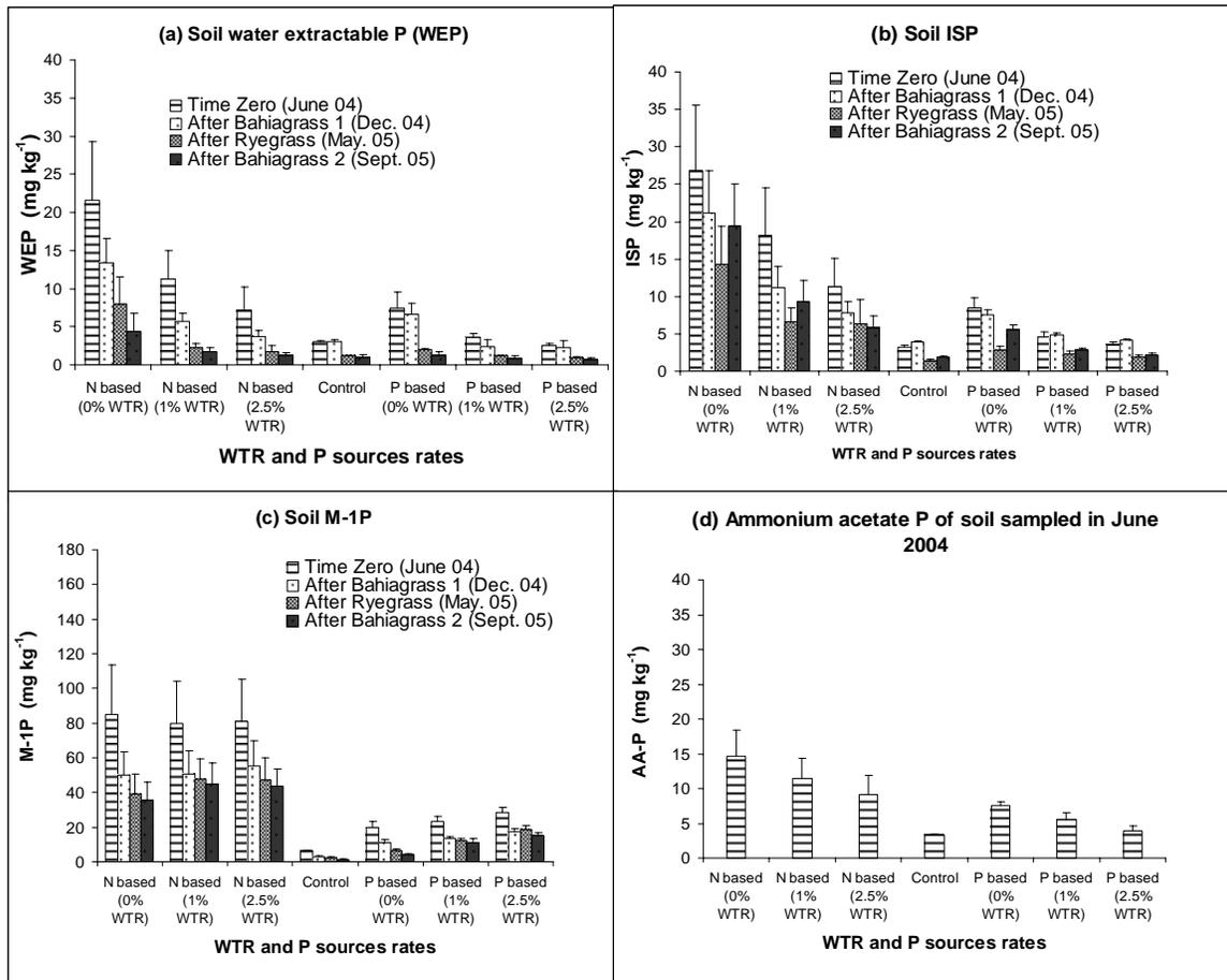
Figure 5-1. Extractable P [(a)water extractable P (WEP), (b) iron strip P (ISP), (c) Mehlich 1 P (M-1P), and (d) ammonium acetate P (AA-P )] values in samples taken during the glasshouse study as affected by application rates of P-sources and water treatment residual (WTR). Note the different scale for M-1P
