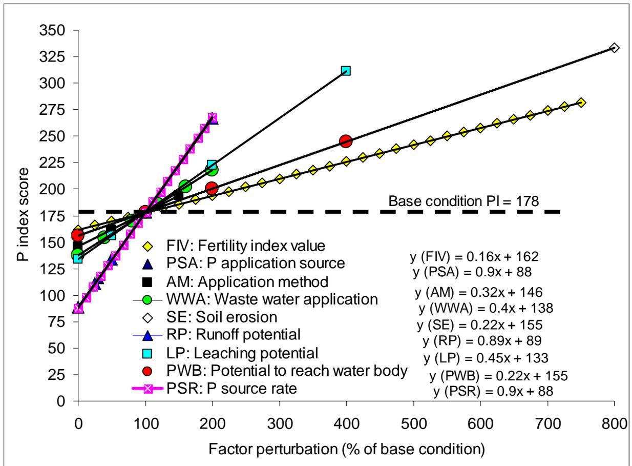
Figure 10-2. Spider diagram of variables in the draft Florida P Index.
