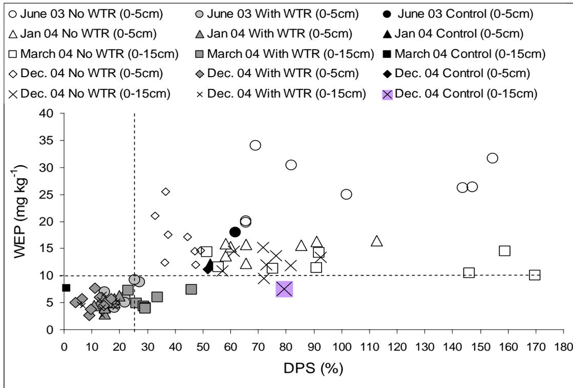
Figure 4-6. Soil water extractable P (WEP) values as affected by degree of P saturation (DPS) values of soil samples taken between June 2003 and December 2004 (Vertical dotted line locates the 25% DPS environmental threshold).
