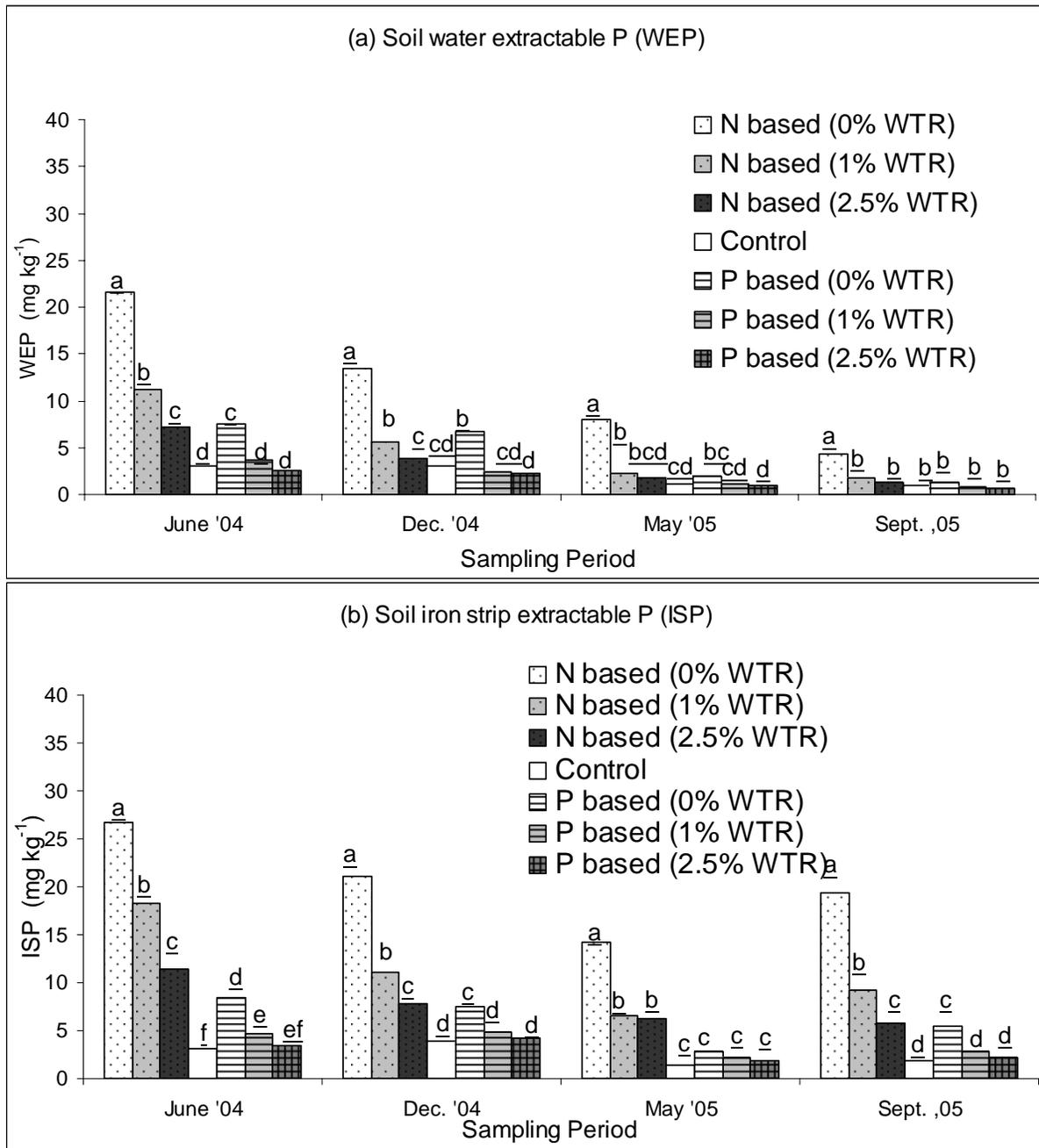
Figure 3-4. Effects of WTR and P-source rates on (a) water extractable P (WEP) and (b) Iron strip extractable P (ISP) values of soil samples taken during the glasshouse study. Treatments within the same sampling period with same letter are not different at *p*-value of 0.05 by Tukey test.
