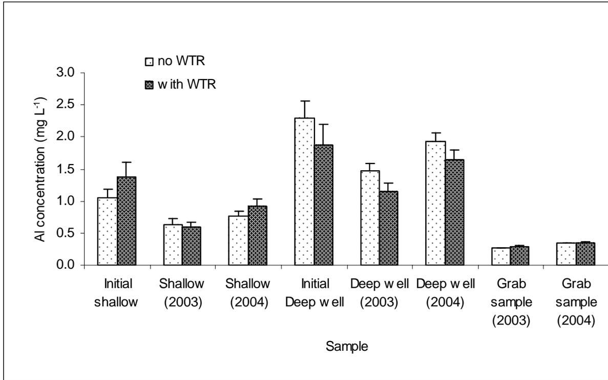
Figure 9-6. Aluminum concentrations in water samples taken during the study as affected by surface applied WTR (n = 24, error bars represent one standard error).
