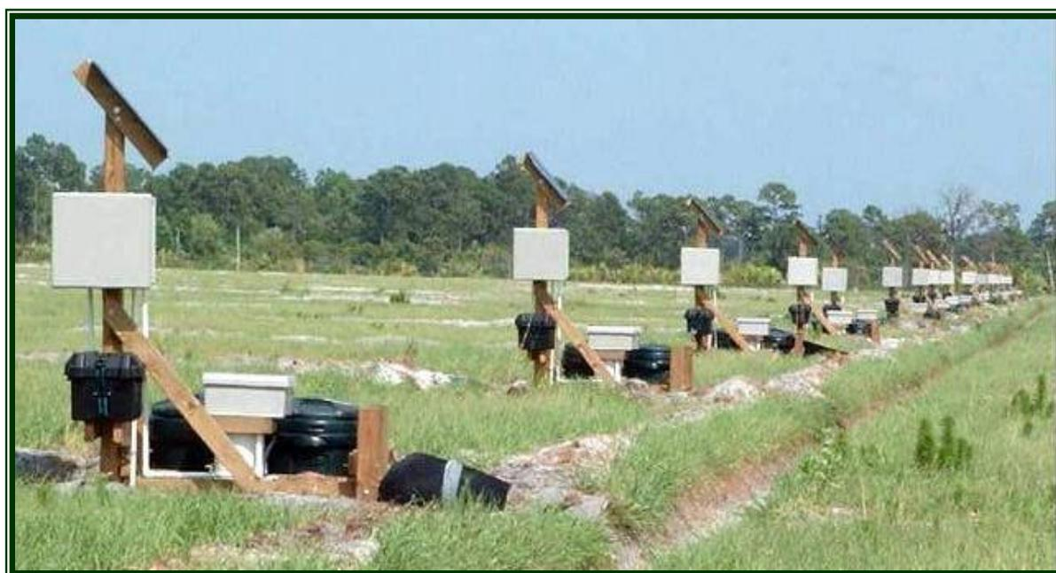
Figure 9-3. One of the experimental blocks (replicates) showing the water sampler and the telemetry installed on each of the 17 rows of plots in the field study.
