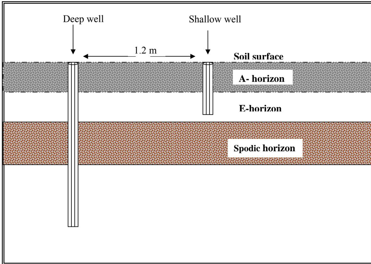
Figure 9-1. Deep and shallow well positions under ground in the field study
