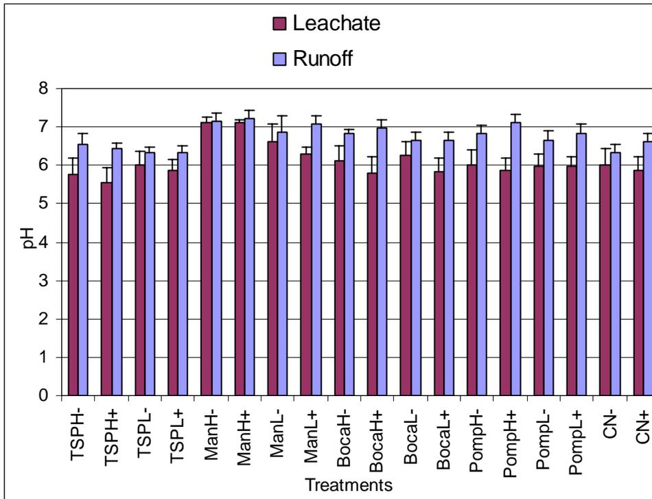
Appendix Figure B-4. Runoff and leachate pH values of the treatments across the three runs and replicates during the rainfall simulation experiment (n = 6, error bars represent one standard error)
