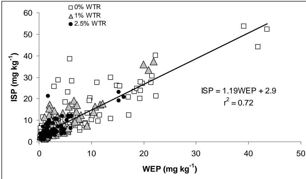
Figure 5-5. Regression of water extractable P (WEP) and iron strip P (ISP) values of soils sampled at planting of the three croppings..
