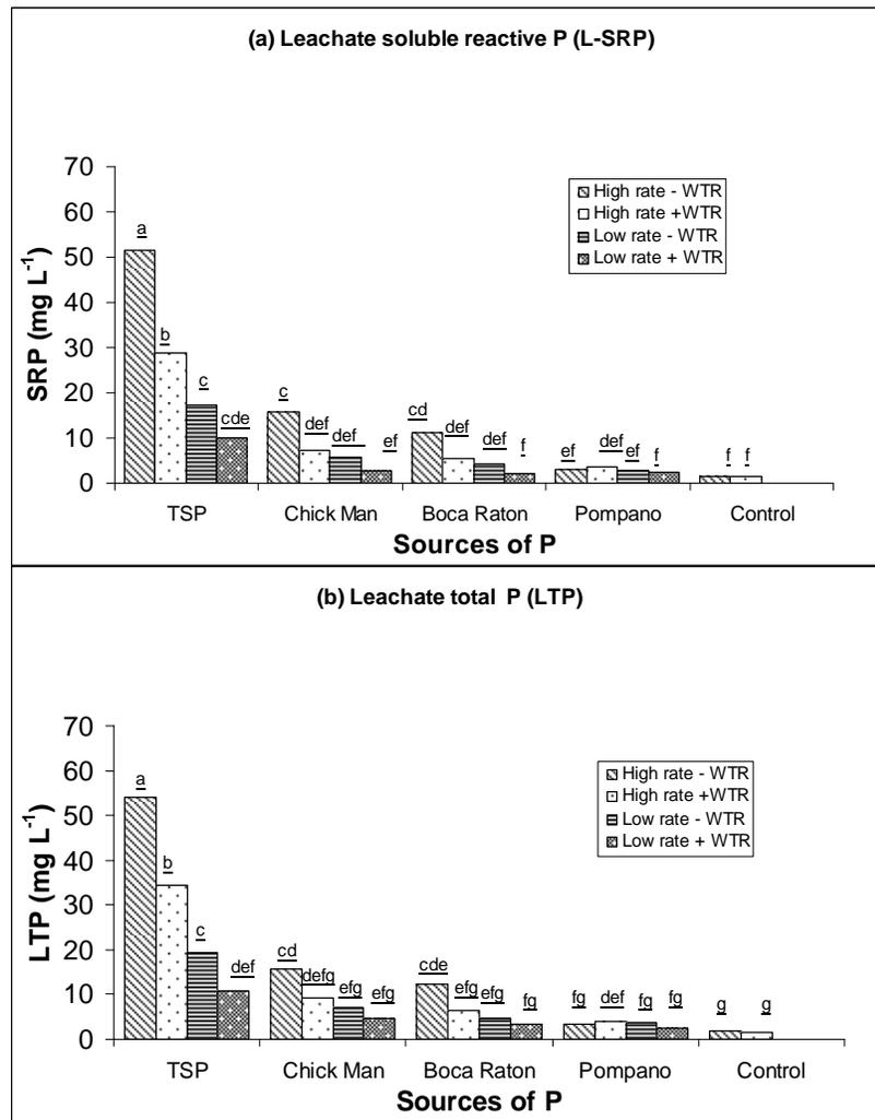
Figure 7-2. Leachate flow-weighted mean (a) soluble reactive P and (b) Total P concentrations for the various treatments. (Treatments bars capped by the same letters are not different at  $p = 0.05$  by Tukey)
