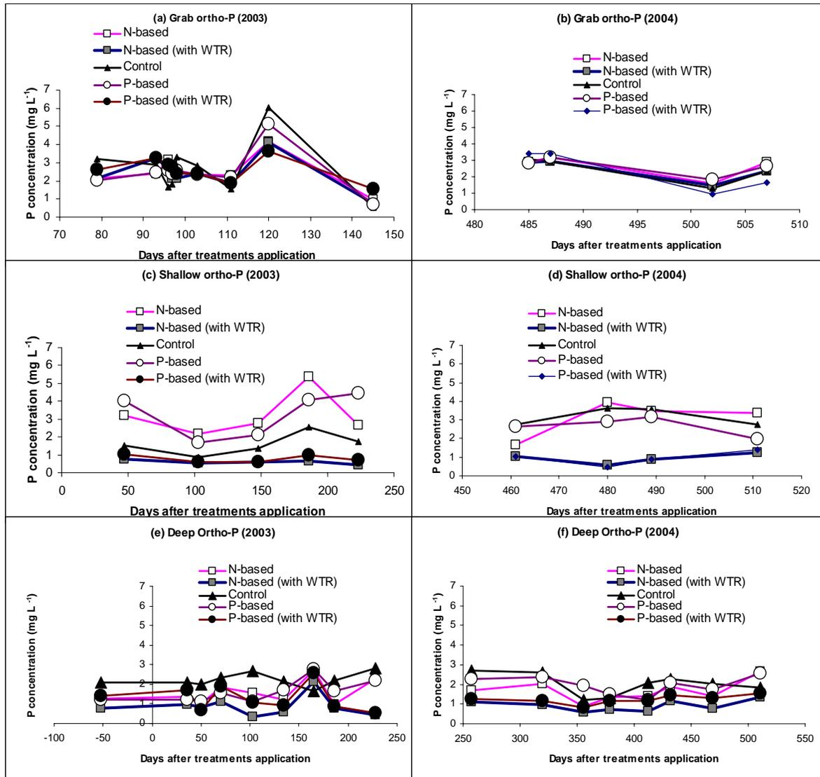
Figure 9-8. Trends of ortho-P concentrations for the various treatments in surface grab (a and b), shallow well (c and d) and deep well (e and f) water samples taken during the study. (Note: Data for “pre-application” shallow well samples are pending in the lab as of the time of this report, and no surface grab samples were taken until 130 days after treatment application).
