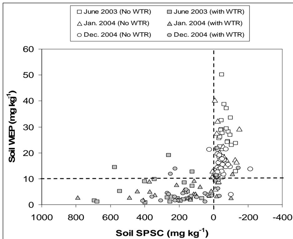
Figure 6-5. The soil phosphorus storage capacity (SPSC, mg kg<sup>-1</sup>) and water extractable P (WEP, mg kg<sup>-1</sup>) values of soil samples obtained from the A horizon (0-5cm) during the field study.
