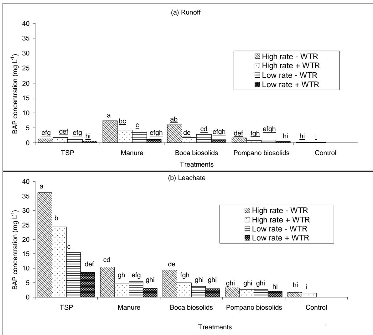
Figure 7-4. Flow-weighted (a) runoff and (b) leachate bioavailable P (BAP) concentrations for the various treatments (Treatments bars capped by the same letters are not different at  $p = 0.05$  by Tukey).
