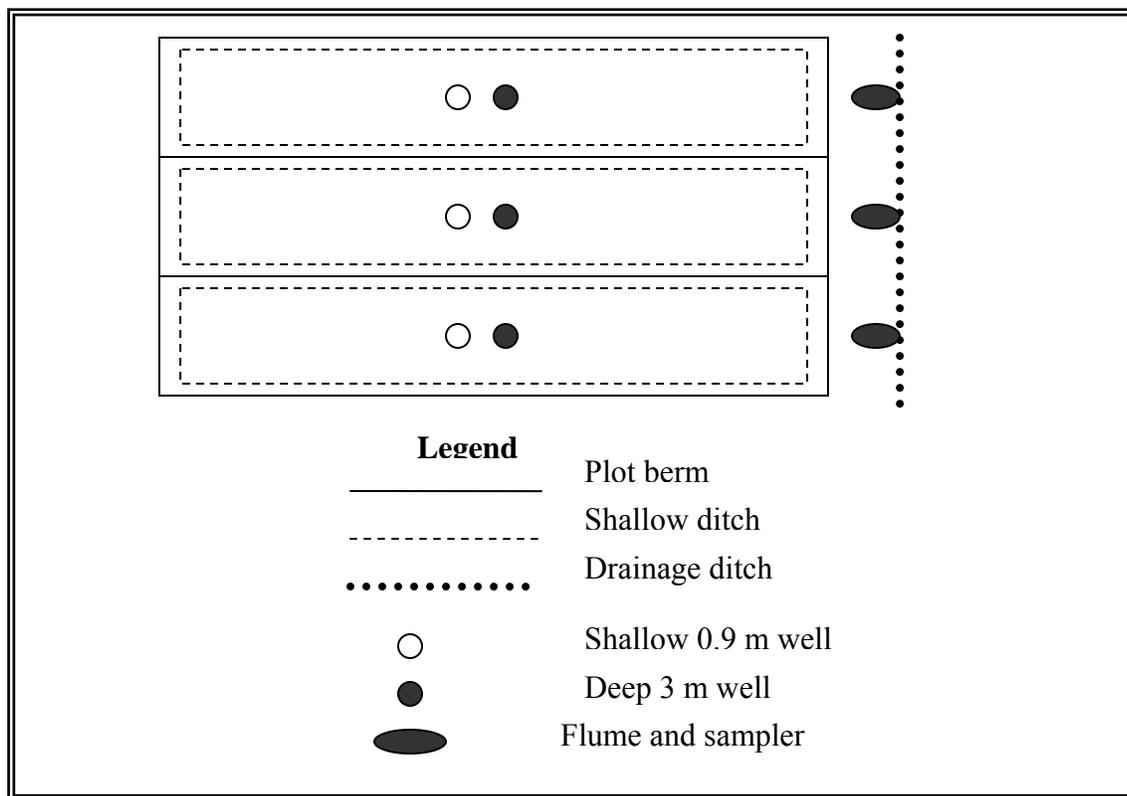
Figure 9-2. Plot layouts and water samplers locations in the field study
