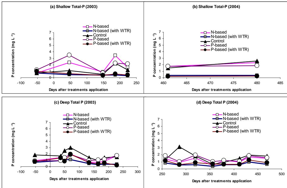
Figure 9-9. Trends of total dissolved P concentrations for the various treatments in shallow (a and b), and deep well (c and d) water samples taken during the study
