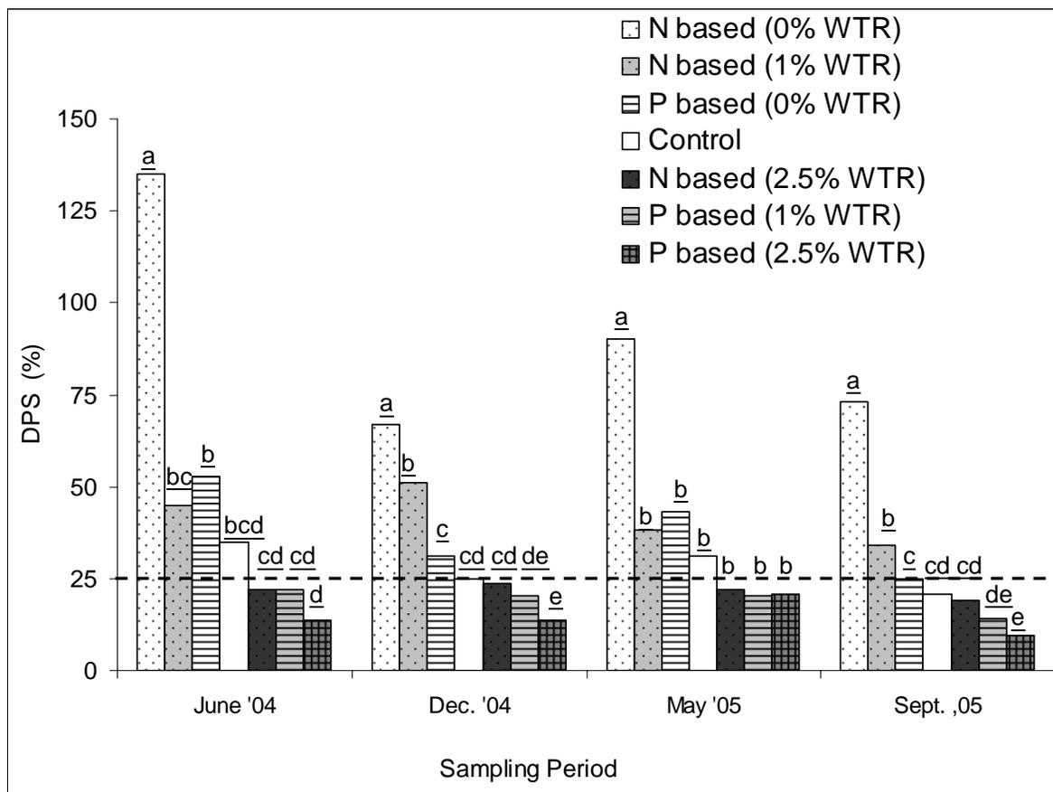
Figure 3-6. Effects of WTR and P-source rates on degree of P saturations (DPS) values of soil samples taken during the glasshouse study. (Treatments within the same sampling period with by the same letter are not different at 5% significant level by Tukey test). Dotted line represents 25% threshold DPS value.
