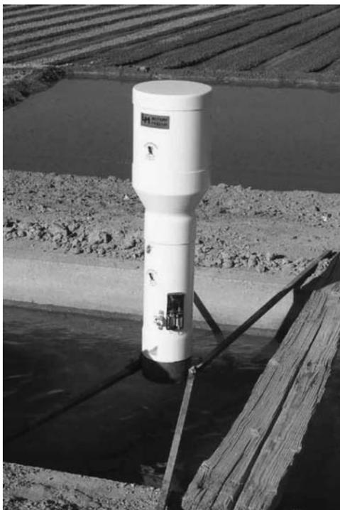
**Fig. 1.** Battery-powered, rotary feed polyacrylamide (PAM) applicator dosing inflow water.
