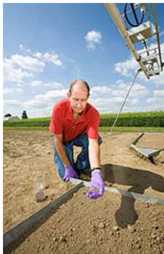
Soil scientist Darrell Norton applies pelletized gypsum and polyacrylamide (PAM) to a soil surface to control erosion prior to a rainfall-simulation test.
