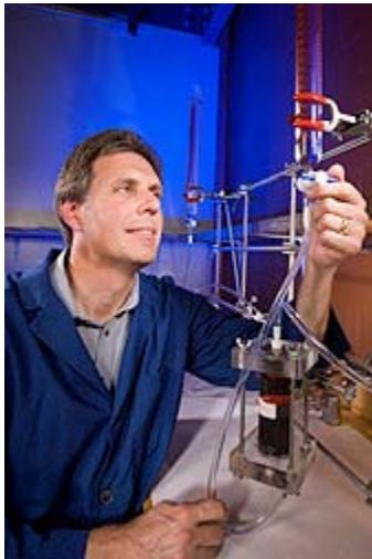
Agricultural engineer Barry Allred conducts an experiment to measure permeability (water flow capacity) of a filter material.
