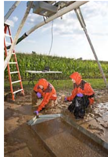
Technician Brenda Hoffman and Samuel Beskow, visiting scientist from the Federal University of Lavras, Brazil, collect sediment to quantify effectiveness of erosion control obtained with pelletized gypsum and polyacrylamide. (D1321-1)
