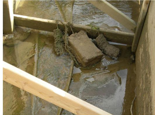
Figure 3: CaCO<sub>3</sub> Blinding of the Floc Log
