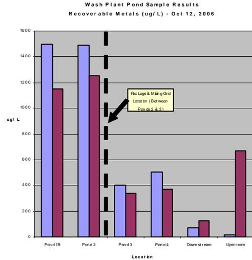
Figure 9: Ponds 1 – 4 & Downstream / Upstream Aluminum & Iron
