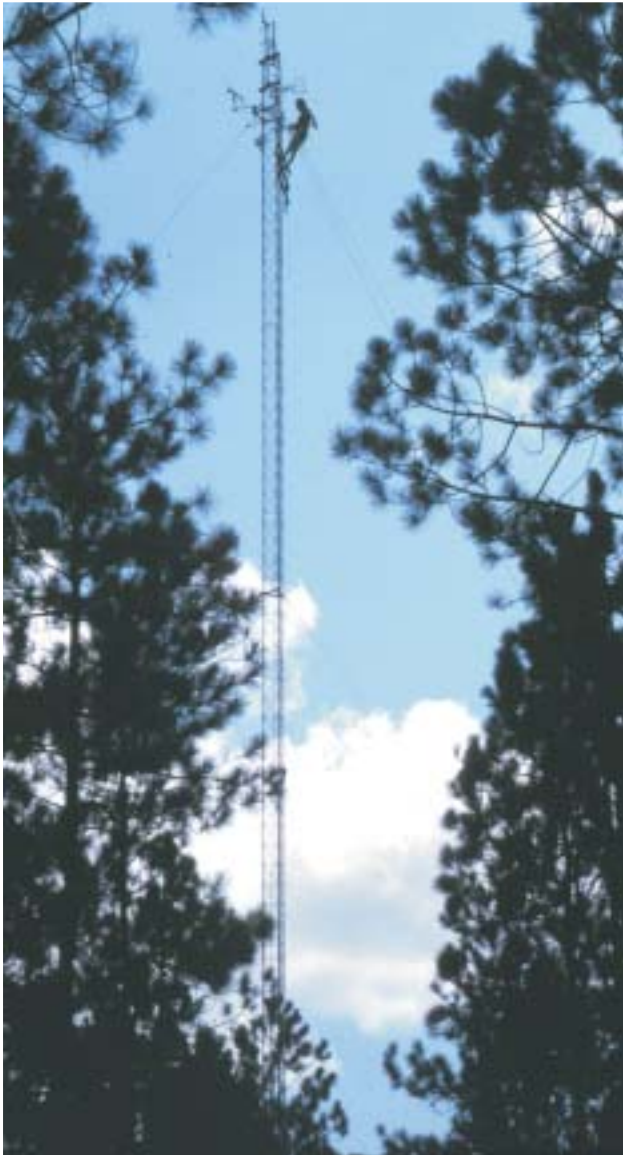
Figure 6. Evapotranspiration station being serviced by hydrologic technician.
