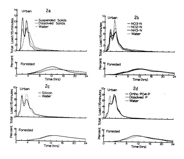
Figure 2: Comparison of the percent total loads of water, suspended and dissolved solids (2a), dissolved inorganic nitrogen species (2b), dissolved silicon (2c) and dissolved phosphorus (2d) transported in 15 minutes versus time for the two experimental watersheds for storm of November 21, 1973. Modified after Turner et al. (22).
