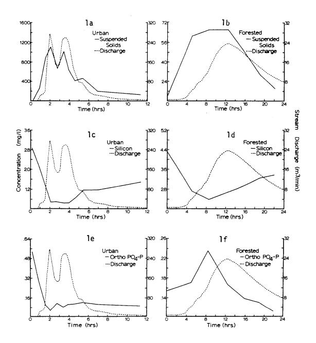
Figure 1: Comparison of stream discharge and concentrations of suspended solids, silicon, and ortho phosphate-phosphorus (PO<sub>1</sub>-P) versus time in the two experimental watersheds for storm of November 21, 1973. Note variations in horizontal (time) and vertical (discharge and concentration) scales between watershed. Modified after Turner et al. (22).
