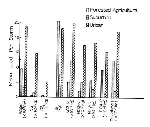
Figure 3: Comparison of mean load per storm for the three watersheds.
