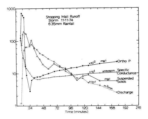
Figure 4: Comparison of discharge of water and concentrations of ortho phosphate-phosphorus, specific conductance, and suspended solids in shopping mall runoff at Tallahassee, Florida.
