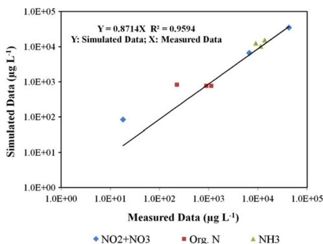
**Fig. 5** Correlation between the measured and simulated values in model calibration
